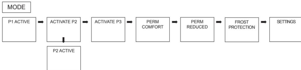
➤ Use **<-** or **->** to scroll through menu points, select desired program and confirm by pressing **OK**.
